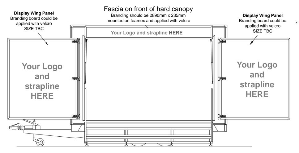
Overall length when full deployed 5520mm Overall width 3550mm including canopy
